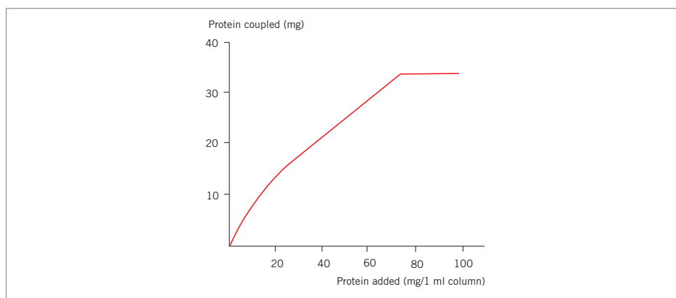
Fig. 60. Ligand coupling to HiTrap NHS-activated HP.
