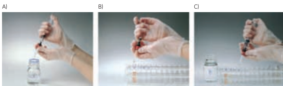
Fig 7.1. Using HiTrap columns with a syringe. (A) Prepare buffers and sample. Remove the column's top cap and twist off the end. (B) Equilibrate the column, load the sample, and begin collecting fractions. (C) Wash and elute, continuing to collect fractions. This procedure is particularly suitable for purification of tagged proteins, because a single step is expected to give a high degree of purification.
