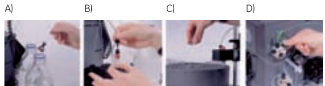
Fig 7.14. Typical procedures using ÄKTAprime plus. (A) Prepare the buffers. (B) Connect the column. (C) Prepare the fraction collector. (D) Load the sample and press start.
