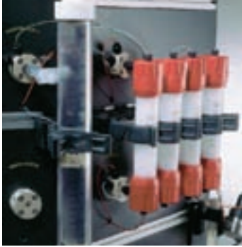
Fig 3.4. A 60 ml sample volume can be desalted on four HiPrep 26/10 Desalting columns connected in series.
